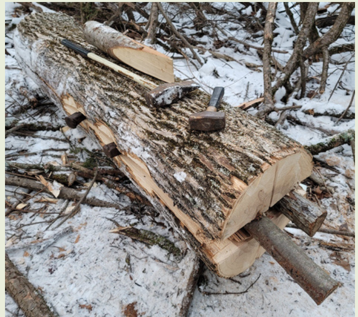
Figure Horizontal Split2: As split progresses, move steel and wooden wedges into the split down the sides. Large wooden wedges in the face open it wider. But, easy does it!
