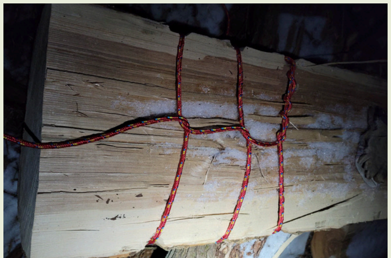
Figure Results: Quality of surface is a function of care in splitting and the grain of the log, with zero knots in this one. The Timber Hitch provides for dragging.
