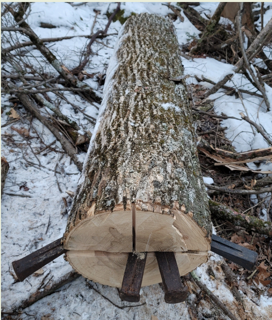
Figure Horizontal Split1: You can use saw cuts (shallower than these) to help start wedges in the face. Also start wedges in corners. Advance by striking wedges in turn.
